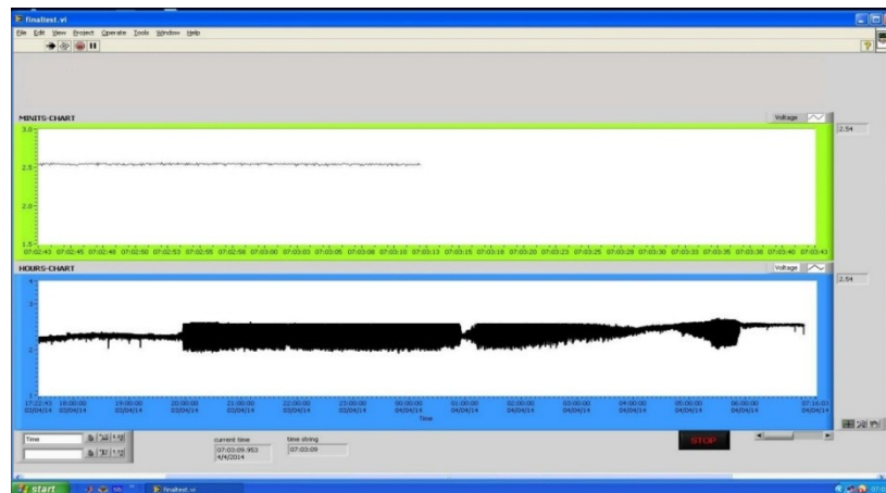
Figure 7(a) : Window of Amplitude scintillation using LabVIEW GUI system
